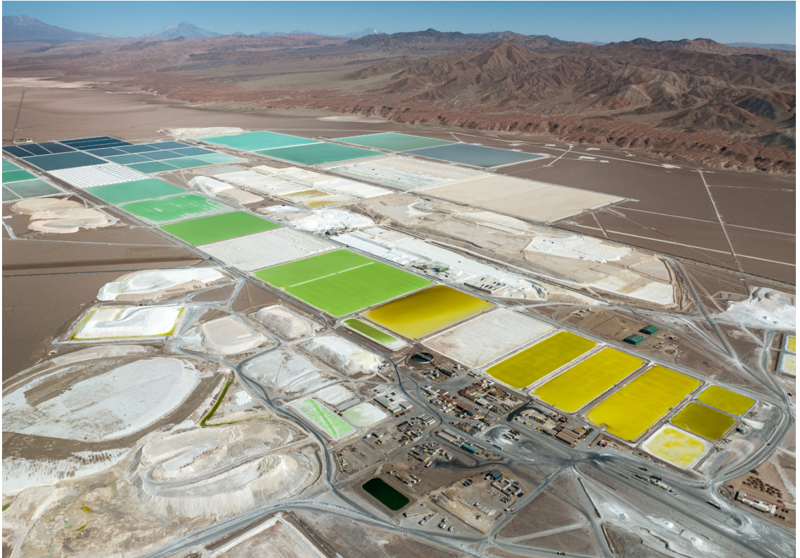
Some lithium mines use immense evaporation ponds to concentrate the metal, demanding excessive land and water. But new technologies may allow for more efficient extraction. Image: John Moore/Getty Images
